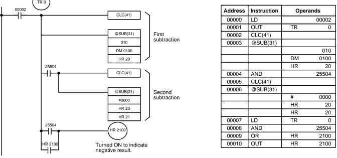
The first and second subtractions for this diagram are shown below using example data for 010 and DM 0100.
